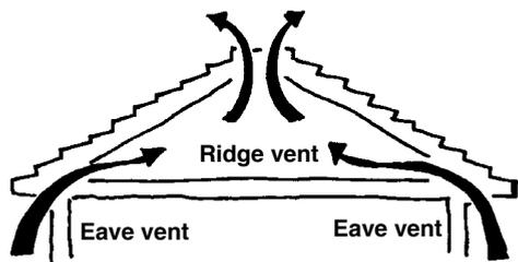
**A combination of ridge and eave vents creates natural convection current, keeping your attic cool and moisture-free.**
