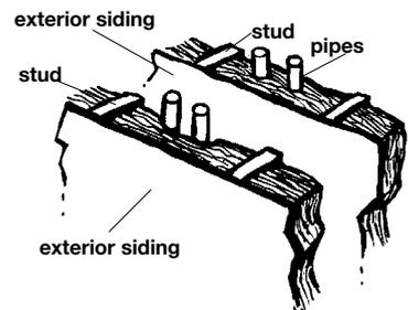
**WHEN INSULATING OPEN SIDE WALLS, BE SURE TO PLACE INSULATION BETWEEN PIPES AND OUTSIDE WALLS.**
