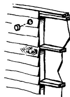
**AFTER INSULATING, THE CONTRACTORS WILL PLUG THE HOLES AND/OR REMOUNT THE SIDING.**
