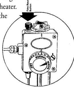
2. Depress the indicator knob and light the pilot. (Continue holding the indicator knob for one minute after the pilot is lit. The pilot flame should remain on when the knob is released.)
