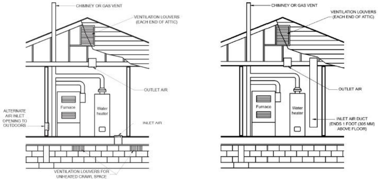
Where directly communicating with the outdoors, or where communicating with the outdoors through vertical ducts, each opening shall have a minimum free area of 1 square inch per 4,000 Btu/h of total input rating of all appliances in the enclosure. ( Total BTU Input of all Appliances / 4,000 = Total Free Area Required )
