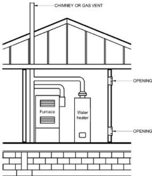
Each opening shall have a minimum free area of 1 square inch per 1,000 Btu/h of the total input rating of all appliances in the space, but not less than 100 square inches. ( Total BTU Input of all Appliances / 1,000 = Free Area Of Each Opening Required )
