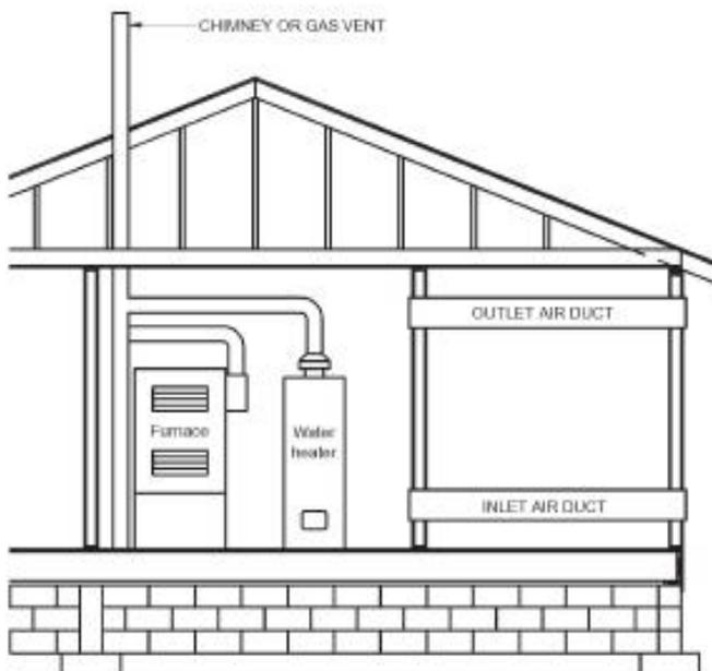
Where communicating with the outdoors through horizontal ducts, each opening shall have a minimum free area of not less than 1 square inch per 2,000 Btu/h of total input rating of all appliances in the enclosure. ( Total BTU Input of all Appliances / 2,000 = Total Free Area Required )
